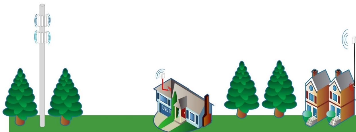
Figure 23: Example Fixed Wireless Network with Access Point Antennas on a Monopole
